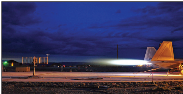
Figure 4. NAH measurement array positioned approximately 50 feet downstream during a nighttime F-22 afterburner engine power run.
